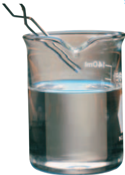
A seed crystal of sodium acetate is added to a supersaturated solution of sodium acetate.
