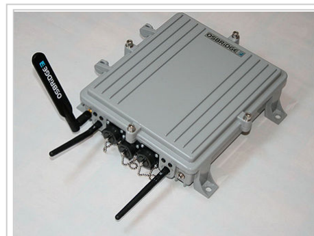
OSBRiDGE 3GN – 802.11n Access Point and UMTS/GSM Gateway in one device
