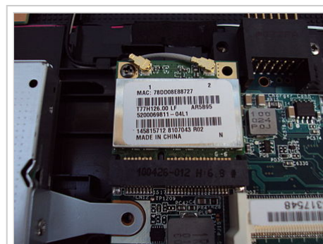
An Atheros draft-N Wi-Fi adapter with built in Bluetooth on a Sony Vaio E series laptop
